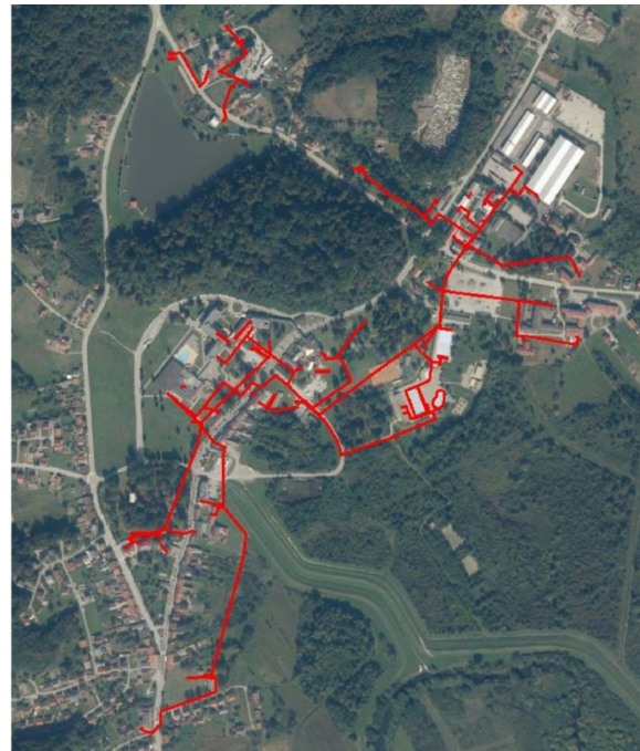
Figure 39 Current structure of DHN in Topusko
